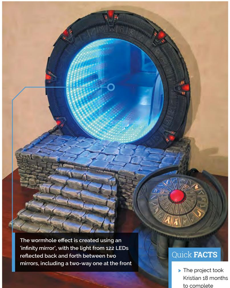
The wormhole effect is created using an 'infinity mirror', with the light from 122 LEDs reflected back and forth between two mirrors, including a two-way one at the front
