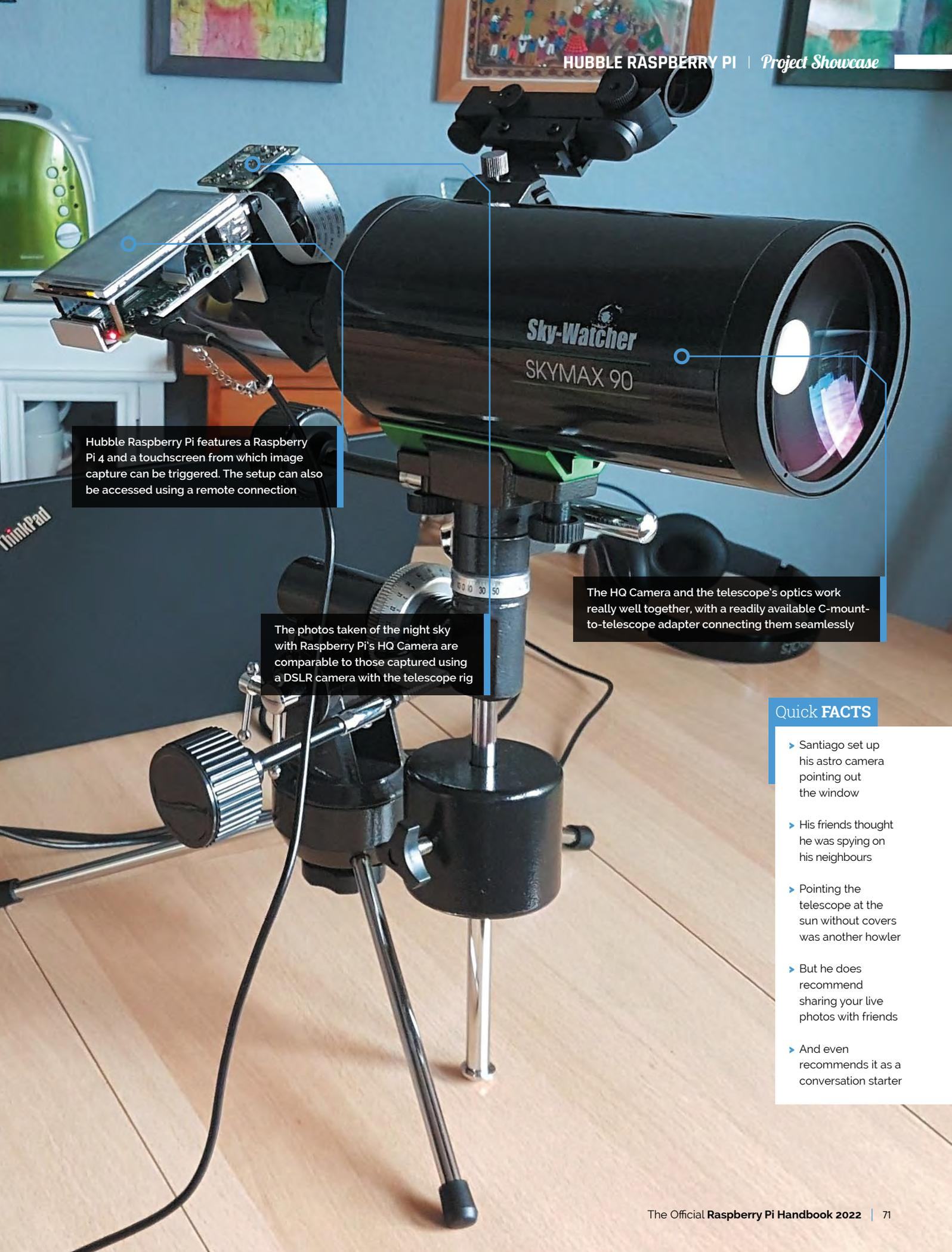
Hubble Raspberry Pi features a Raspberry Pi 4 and a touchscreen from which image capture can be triggered. The setup can also be accessed using a remote connection
