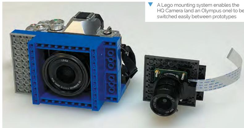
▼ A Lego mounting system enables the HQ Camera (and an Olympus one) to be switched easily between prototypes
