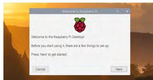
**03 Set up Raspberry Pi** When Raspberry Pi Imager has finished verifying the software, you will get a notification window. Remove the microSD card and put it in your Raspberry Pi. Plug in your Raspberry Pi power supply and, after a few seconds, a blue screen will appear with 'Resizing Filesystem'. It will quickly vanish and be replaced by 'Welcome to Raspberry Pi'. Click on Next and follow the on-screen instructions to set up Raspberry Pi OS and start using your new computer.
