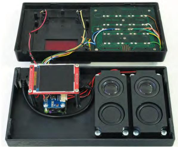
▲ The inner workings include a Raspberry Pi Zero with WM8g60 Audio HAT, speakers, and 176×220 LCD
