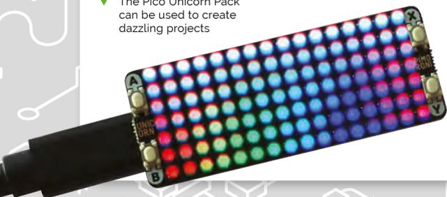
white LEDs. The Unicorn Pack can be used to create a rainbow display for your window ([magpi.cc/rainbow](https://magpi.cc/rainbow)), as well as simple animations. The Scroll Pack can be used to create scrolling text messages (hence the name), and it's also great for displaying graph data and for creating a status light.
