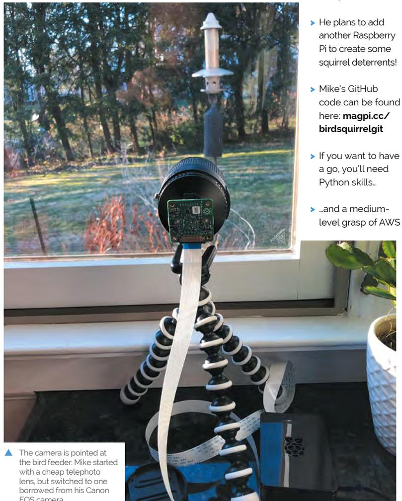
▲ The camera is pointed at the bird feeder. Mike started with a cheap telephoto lens, but switched to one borrowed from his Canon EOS camera
