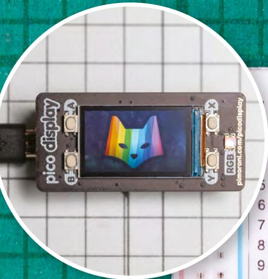
The functionality of Pico can be expanded directly with add-ons such as the Pico Display Pack, which adds a 1.14-inch IPS LCD display and four buttons
