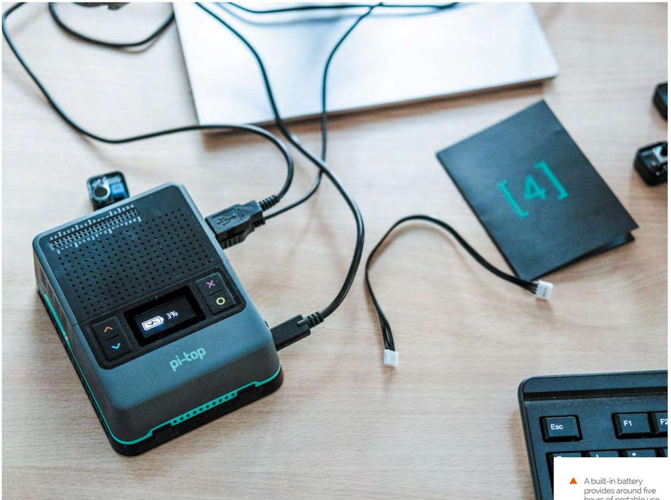
▲ A built-in battery provides around five hours of portable use
