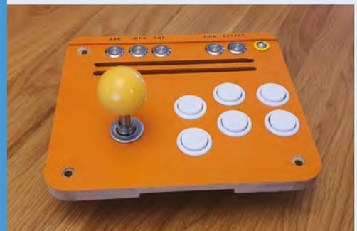
**03** The control block enables the arcade to safely shut down via the power button on the front. Attach it to Raspberry Pi using the GPIO pins.
