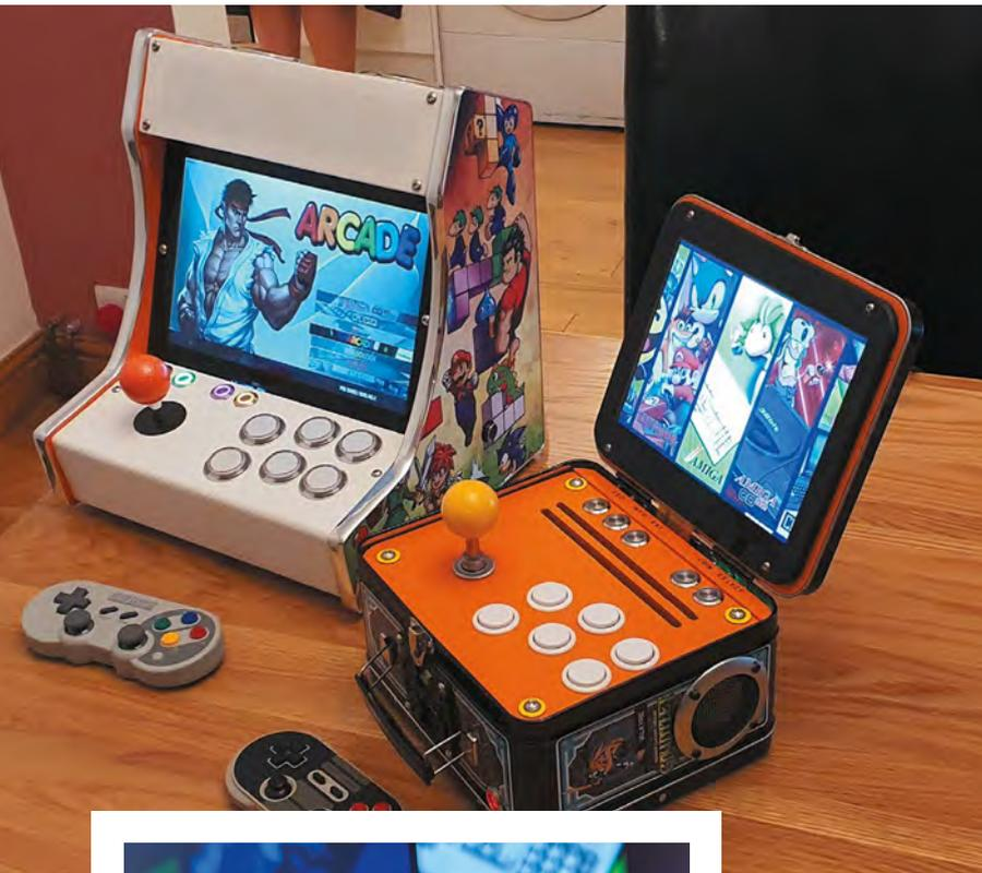
the LCD screen. “I was able to gain some height with new hinges. This allows the screen to fold inside the casing, giving a seamless look when shut,” Rich says. “The joystick is removable to allow the lid to close. It’s a modified Sanwa joystick shaft with a quick release system. The sprung release shaft comes off easily and can be stored in the back of the machine. The original latch holds the lid shut.”
