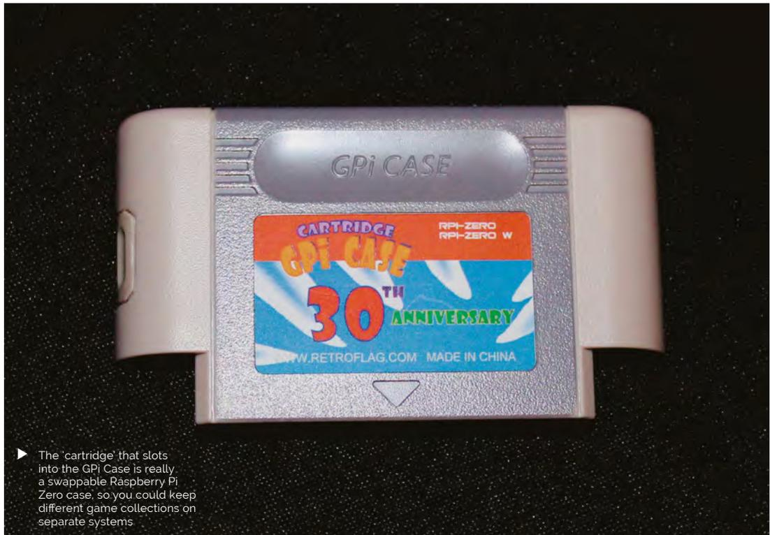
► The 'cartridge' that slots into the GPI Case is really a swappable Raspberry Pi Zero case, so you could keep different game collections on separate systems
