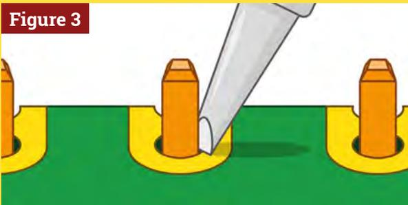
▲ Figure 3 Heat the pin and pad
