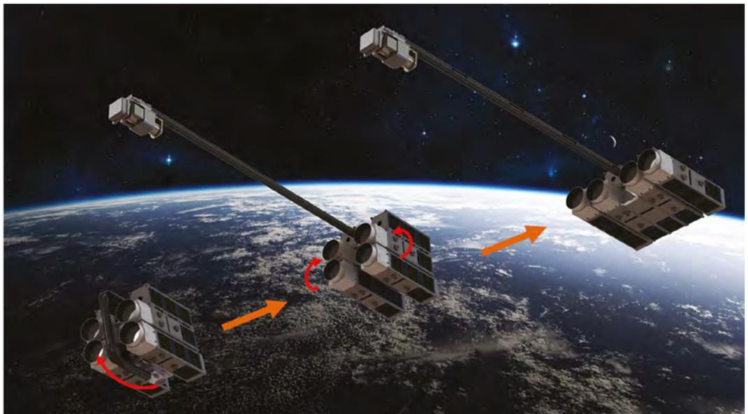
▶ AAReST concept showing how each CubeSat docks to form part of the modular satellite. Credit: AAReST collaboration
