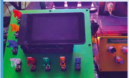
**02** With this data, the computer controls an array of pumps that provide water, nutrients, and pH adjustments. Grow lights are controlled and tweaked, fans are adjusted, heating mats activated, and it even switches between day and night vision for the camera.
