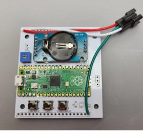
A Raspberry Pi Pico controls it all, shown here mounted on an optional PCB with buttons and a real-time clock module
