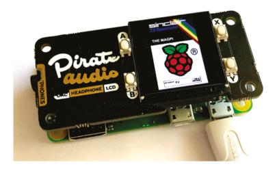
The Pirate Audio HAT is a DAC (digital-to-analogue converter) combined with a small headphone amp battery-powered headphone amp. You need to connect its input to the Pirate Audio HAT and the output to the ZX Spectrum. It will provide the final boost needed for reliable loading.
