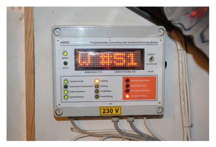
Zsolt's controller allows the user to see at a glance the status of the crop and the current environment settings system shows the status of the lights, fans, humidifier, and watering system – including the pressure, and whether or not the tent door is open. "Measurement, timing, and electrical equipment control is done by a Python-language program that
