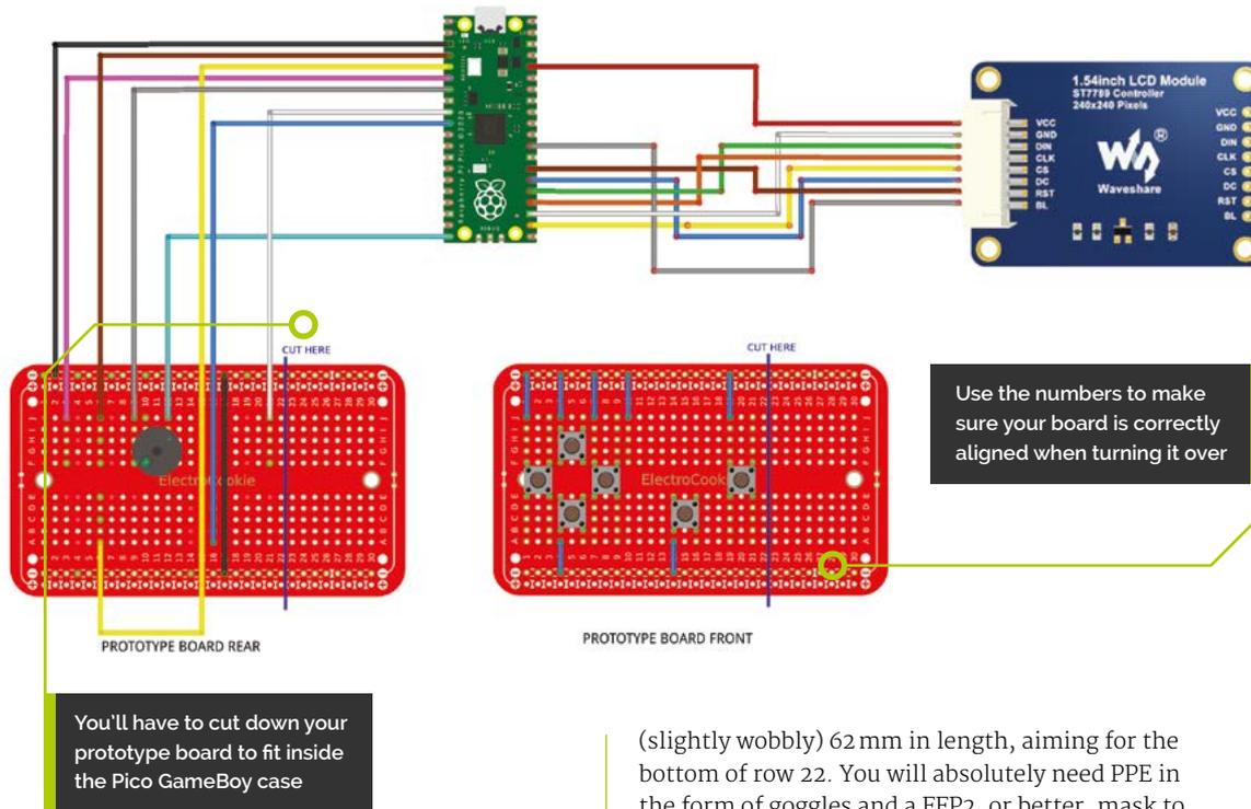
Figure 1 The wiring diagram for the handheld
