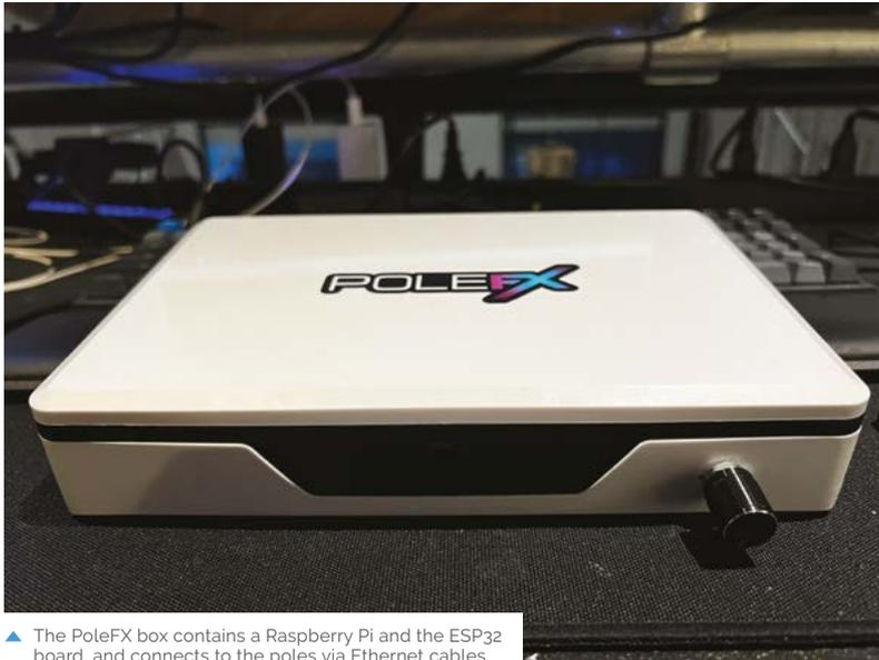
▲ The PoleFX box contains a Raspberry Pi and the ESP32 board, and connects to the poles via Ethernet cables
