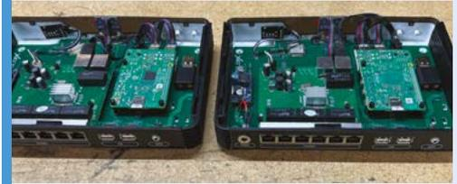
**01** Inside the PoleFX box is a custom ESP32-based board with an Ethernet interface. Each pole is connected to the board via an Ethernet cable which transmits the data to the LEDs.
