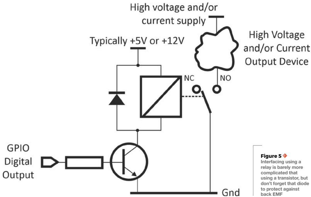
**Figure 5** ♦ Interfacing using a relay is barely more complicated than using a transistor, but don't forget that diode to protect against back EMF
