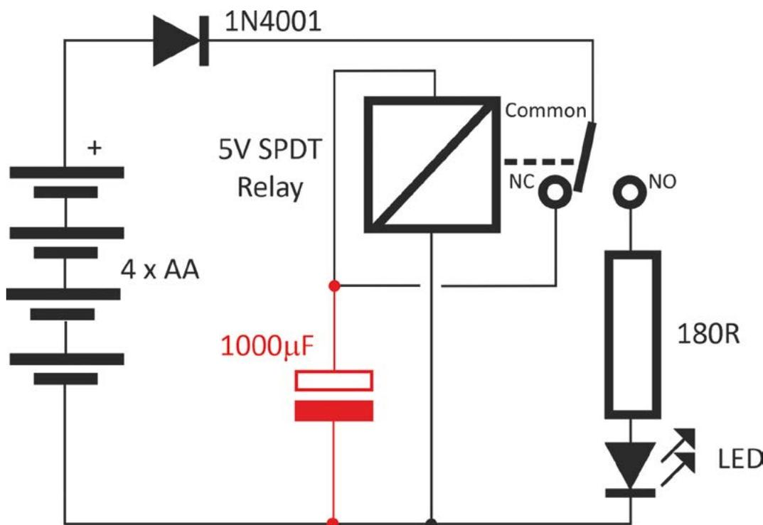
**Figure 2** ♦ We trust you'll be able to see that this circuit will act as an oscillator if the red capacitor is missing. And all you have to know to figure out how the capacitor slows it down is that the capacitor takes a while to charge up, so the relay will take a while to switch once a voltage is applied to it
