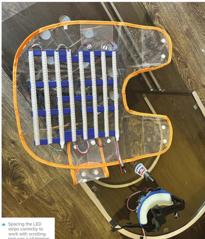
▲ Spacing the LED strips correctly to work with scrolling text was a challenge
