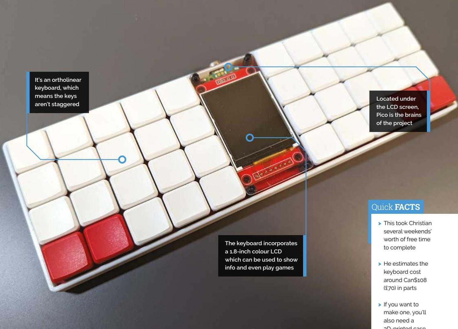
It's an ortholinear keyboard, which means the keys aren't staggered
