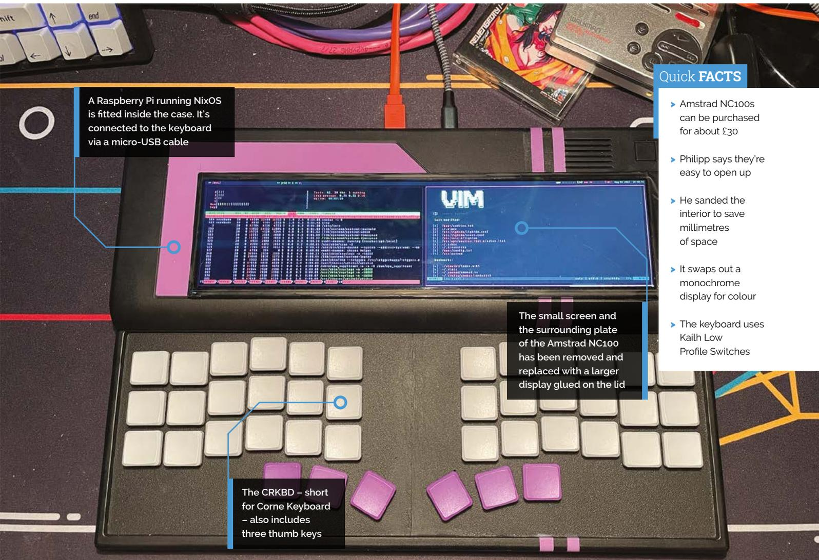
A Raspberry Pi running NixOS is fitted inside the case. It's connected to the keyboard via a micro-USB cable
