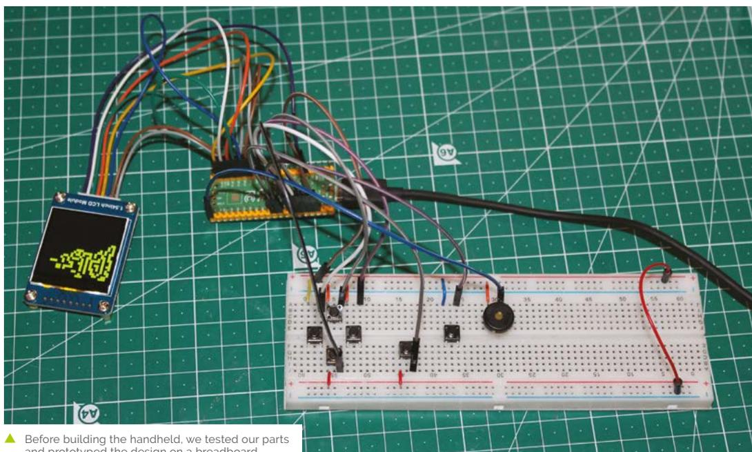
▲ Before building the handheld, we tested our parts and prototyped the design on a breadboard
