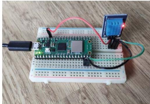
◀ The DHT11 sensor measures both temperature and relative humidity
