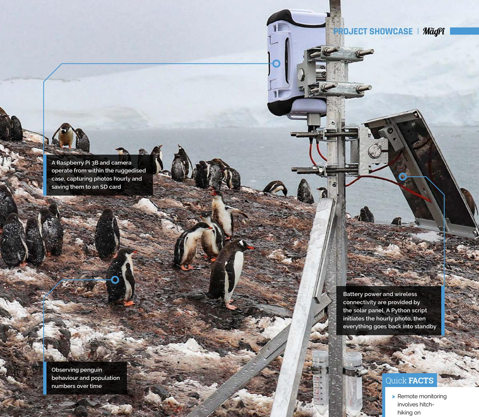
A Raspberry Pi 3B and camera operate from within the ruggedised case, capturing photos hourly and saving them to an SD card
