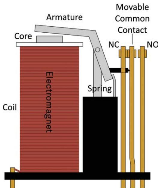
**Figure 1** Understanding how a relay works is a lot easier than getting your head around moving holes and electrons in transistors
