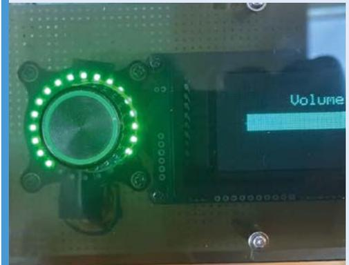
**02** With some hacking, the data is stored and translated to work on the limited VFD via several predetermined screens. The code also looks out for changes in the knobs to know when to display it.
