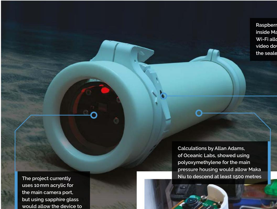
Raspberry Pi Zero is mounted inside Maka Niu and its on-board Wi-Fi allows communication and video download without opening the sealed, watertight unit
