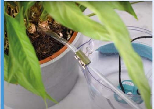
**02** You can download the MicroPython setup code from [magpi.cc/splush](https://magpi.cc/splush) or view the demo video at [magpi.cc/youwatertheplant](https://magpi.cc/youwatertheplant). Once set up, fasten the tube to the edge of the plant pot.
