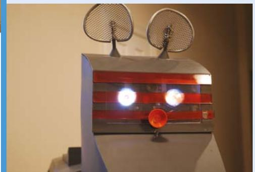
**03** Fitz used Python on his Raspberry Pi 3 to control the camera/printer and eye lights in K-9's head, and to play video clips on K-9's side monitor.
