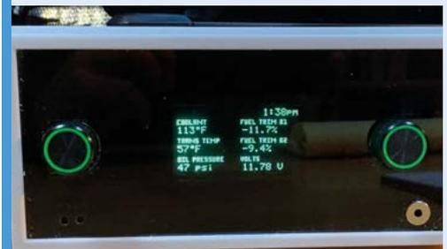
**03** The head unit displays regular information such as the radio, but can be changed for more detailed engine statistics, or even GPS, using the rotary dials like normal knobs. It also maintains the standard Jeep radio aesthetic
