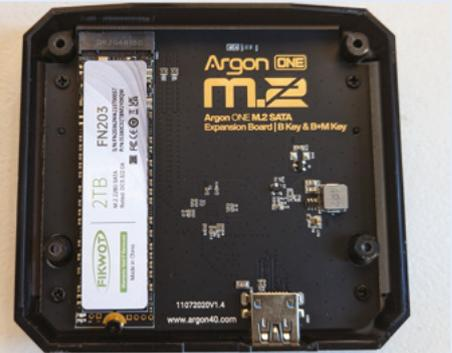
**01** You don’t need many components to copy what Jeffrey made – as well as a Raspberry Pi 4 with at least 2GB RAM, it uses an Argon ONE M.2 case, NanoSound One Hi-Fi DAC, and a 2TB SSD.
