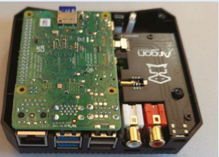
**03** As a 2TB SSD is being used for storage, you only need normal sized SD card for Raspberry Pi. Jeffrey has used 2GB here. The SSD goes into the underside of the Argon ONE case, and connects via a USB 3.0 adapter.
