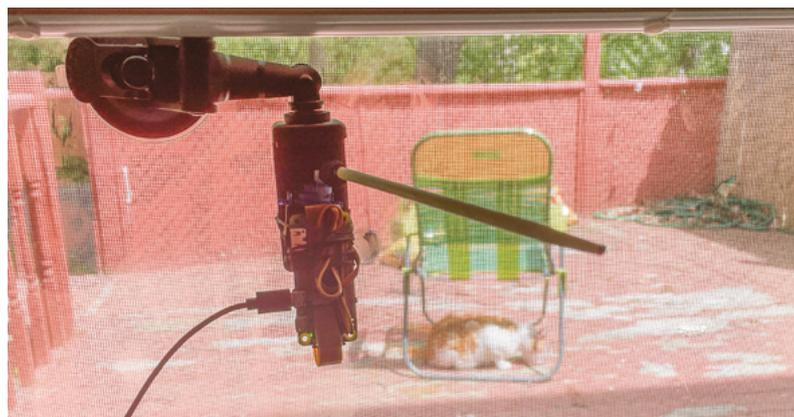
Pi 5 detects a bird, it sends a request to Raspberry Pi Zero to activate the servo.
