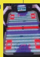
3D-printing and perfecting this 1:5 scale air hockey table. It offers either regular air hockey (first to seven points) or Doom mode for a fiery table lightshow complete with scream effects. Since it uses RetroPie there's also a games emulator mode. The whole crazy caboodle is controlled by Raspberry Pi 4.
