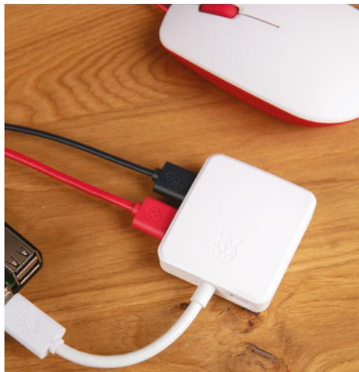
▲ A single upstream USB 3 Type-A connector on 8 cm captive cable connects to Raspberry Pi and provides four downstream USB 3 Type-A ports
