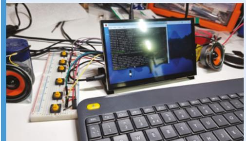
**03** Allie set up buttons to trigger specific songs that were stored on Raspberry Pi and also used Python code to pull tracks from Spotify or YouTube via the Chromium browser that play through the guitar's integrated Bluetooth speakers.
