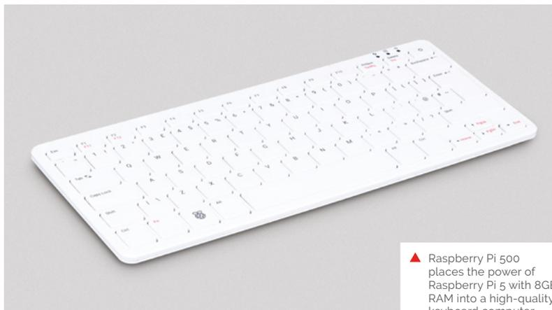
▲ Raspberry Pi 500 places the power of Raspberry Pi 5 with 8GB RAM into a high-quality keyboard computer
